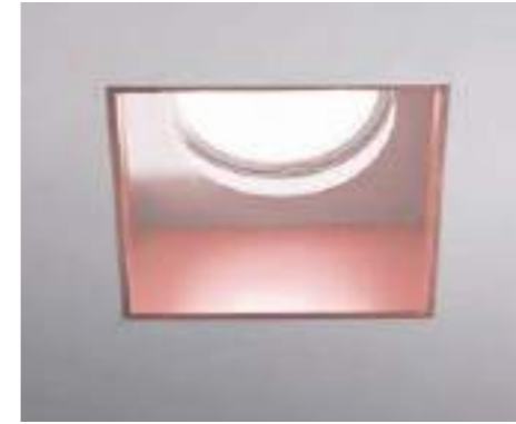
←↓ T417 Elis Raso Flush recessed plaster spotlight with brushed copper finished aluminium frame GU10 x 1x40W w80 x d80 mm aluminium frame
