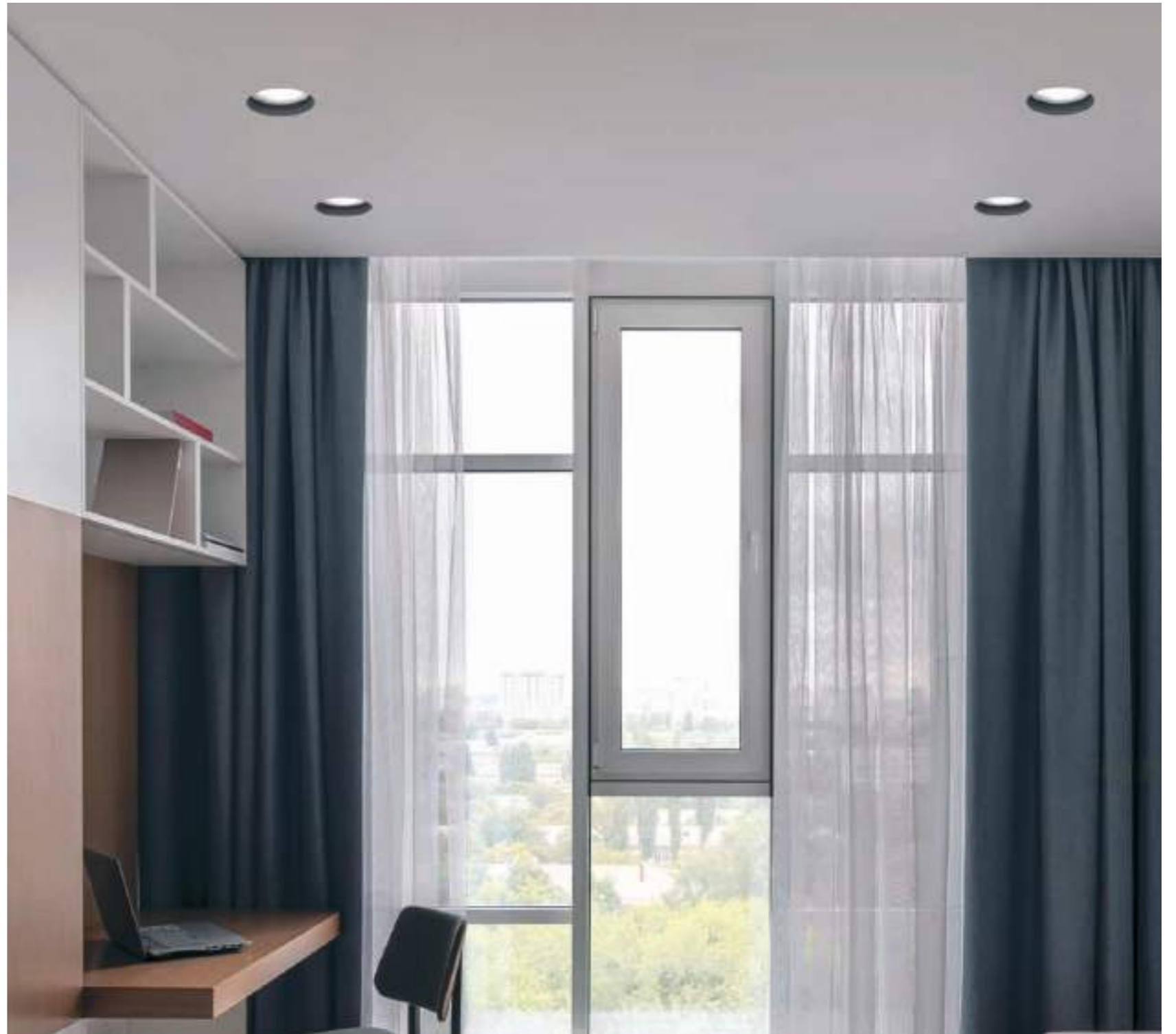
← ↑ T338 Filiatrà Recessed plaster spotlight with black painted inner edge GX53 - 1x10W Ø80 mm lighted hole
